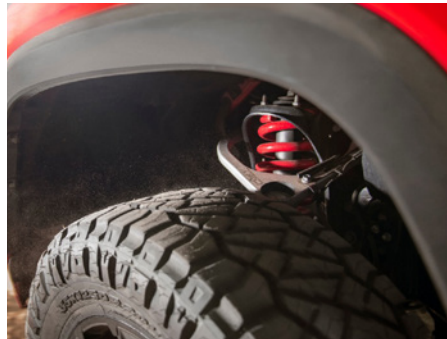
3-in. Suspension Lift Kit 47, 48
